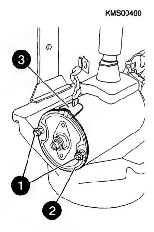
Assembling commutator end shield
